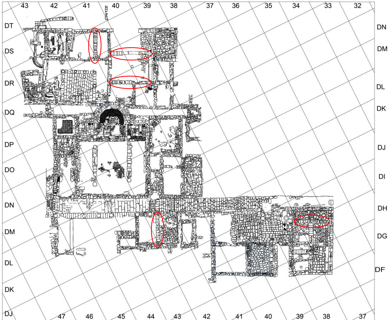
Figure 7: Window walls (circled in red)
